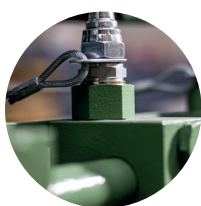
Safety Safety retaining cables on every high-pressure hydraulic pipe
