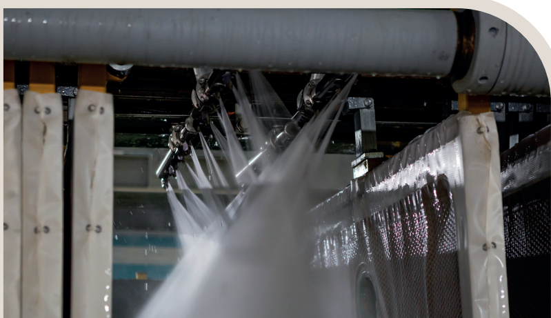
Cloths' washing system equipped with multi-stage centrifugal pump, integrated in the filterpress frame
